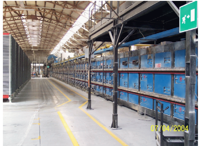
The forno (kiln) at the Omega Factory is HUGE, with temperatures reaching 1000C+ degrees.
