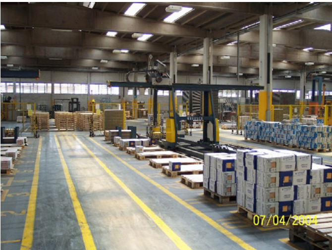
The tile factory runs with approximately 100 employees and robotics, including robotic forklifts that run around the factory moving racks and pallets of tile.
